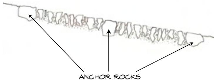
FIGURE 9b. Longitudinal Cross-section of the "Stone Pitching" method of Tread Paving
