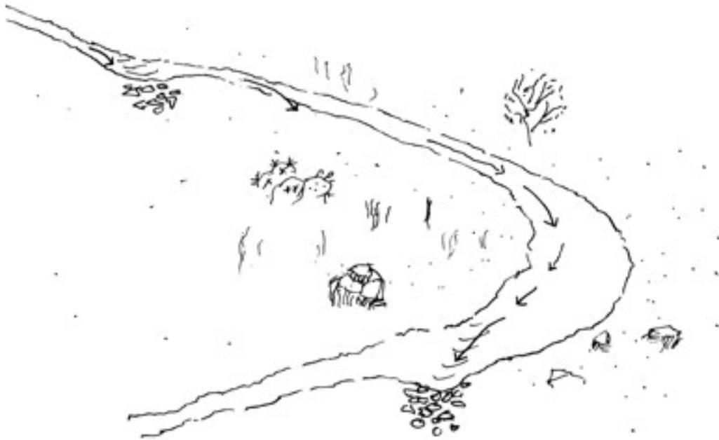
FIGURE 5. Perspective View of Climbing Turn with Drain Dips on Upper Leg and at Bottom of Turn
