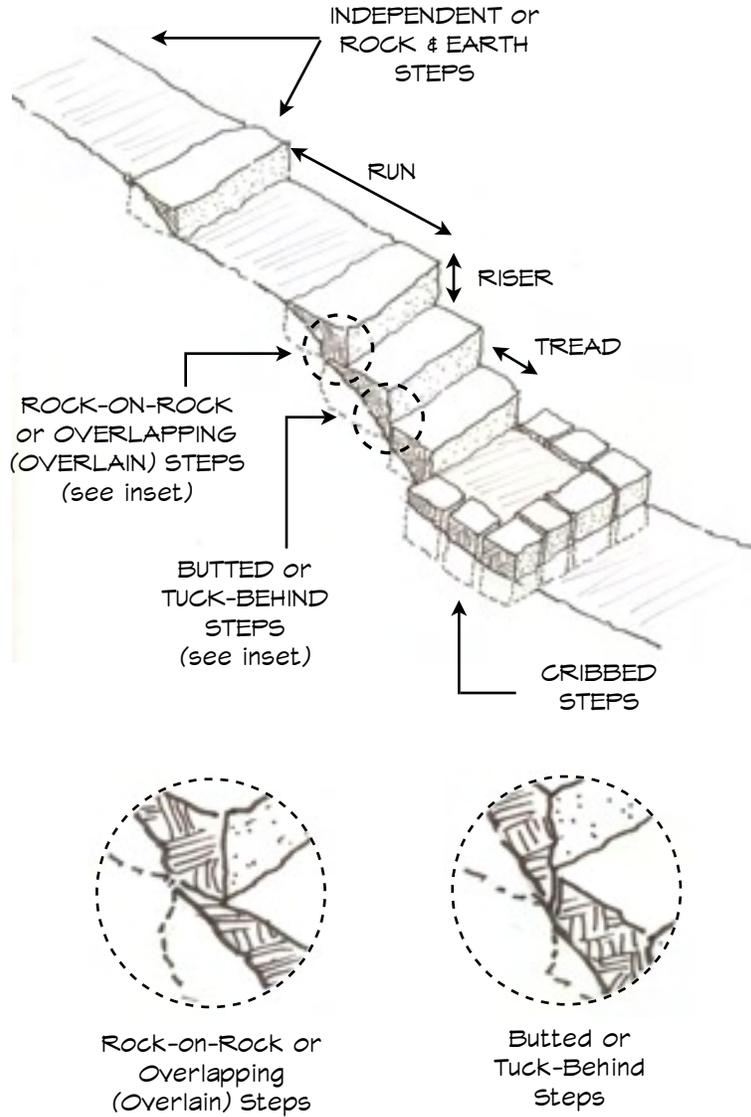
FIGURE 4. Step Components and Configurations
