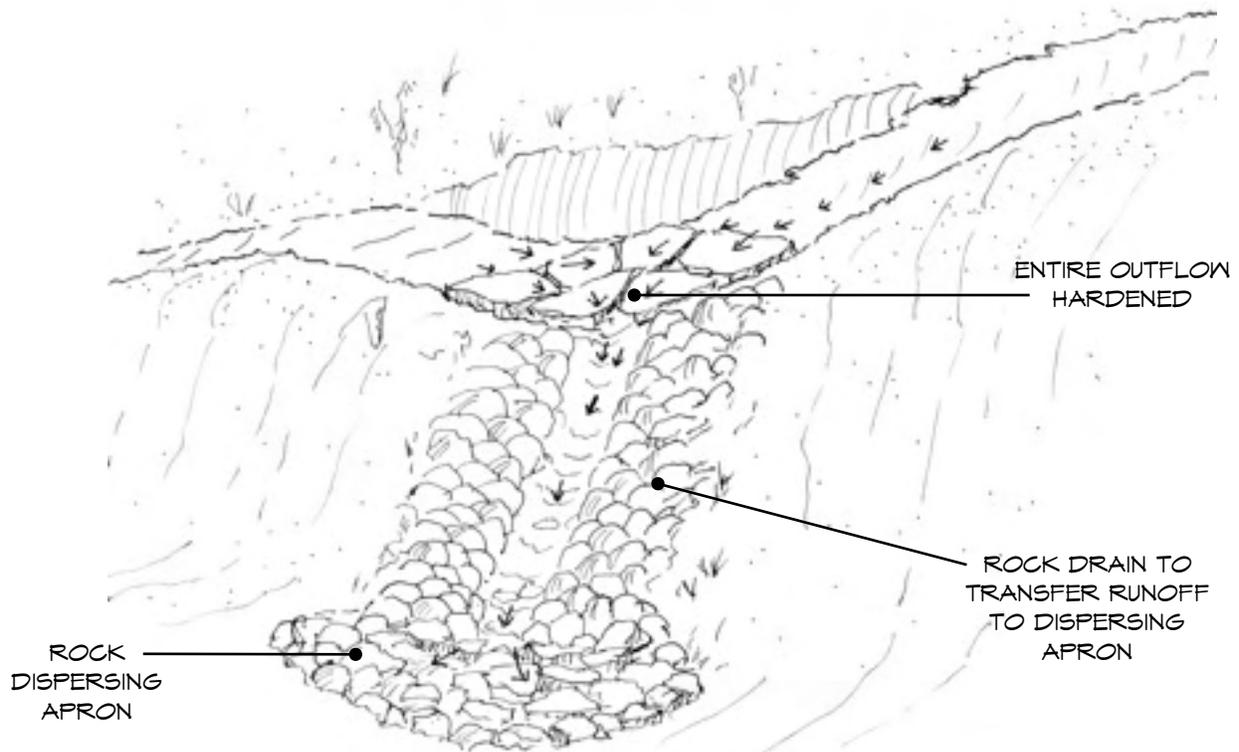
FIGURE 12. Grade Reversal (Drain Dip) with Extensive Hardening
