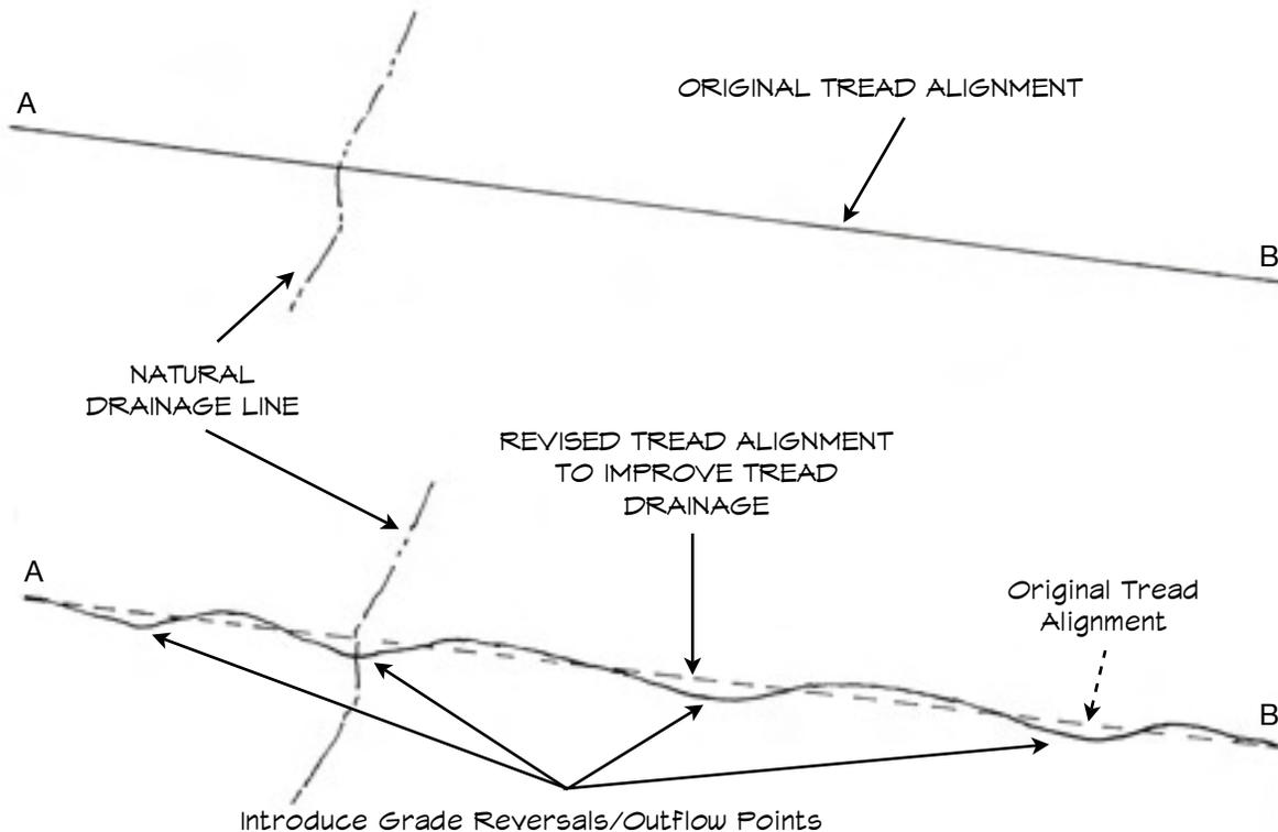
FIGURE 10. Schematic Illustration of Introduced Grade Reversals
