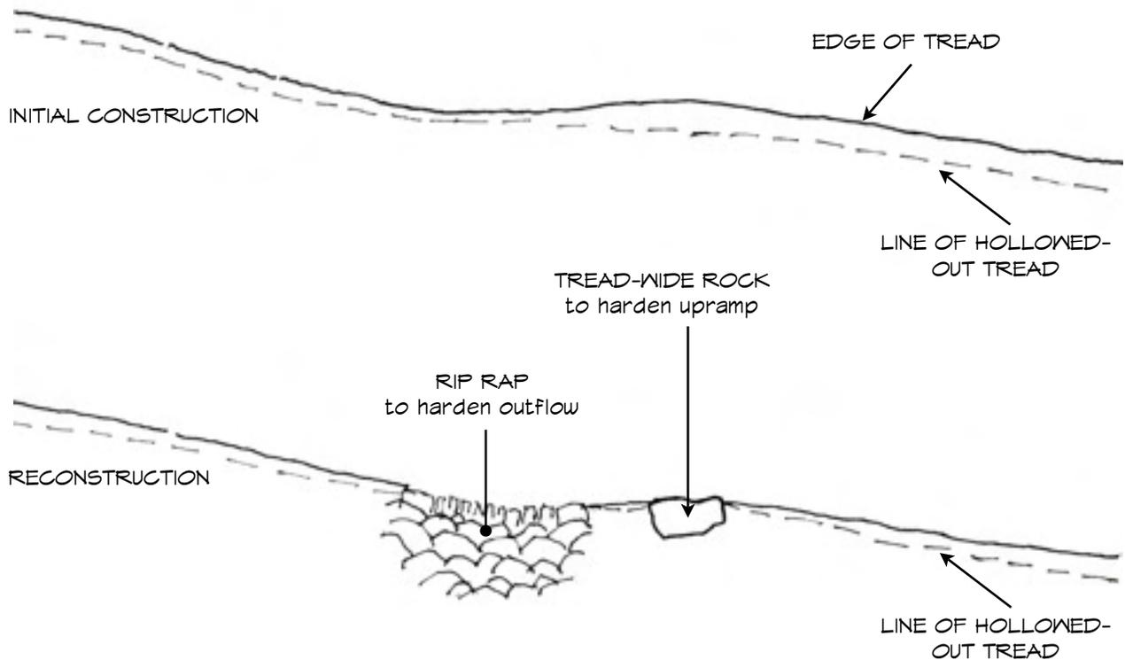
FIGURE 11. Profile View of the Reconstruction of a Hardened Tread
