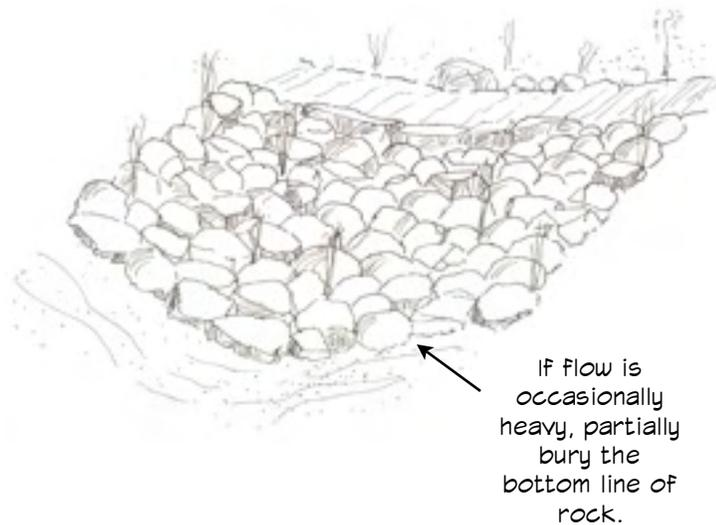
FIGURE 13. One-Rock Dam Below Shallow Drainage Crossing
